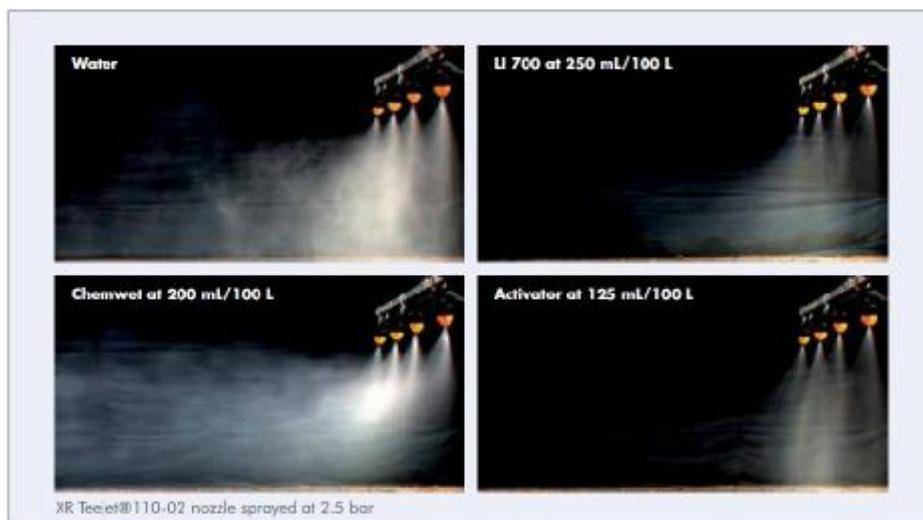
The effect of a spray adjuvant on the amount of drift generated from a nozzle. Note how some non-ionic wetters increase the amount of drift (eg Chemwet) while others can reduce drift (eg Activator).
