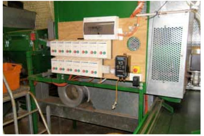
l) *Air sorter for light nut in shell removal*
