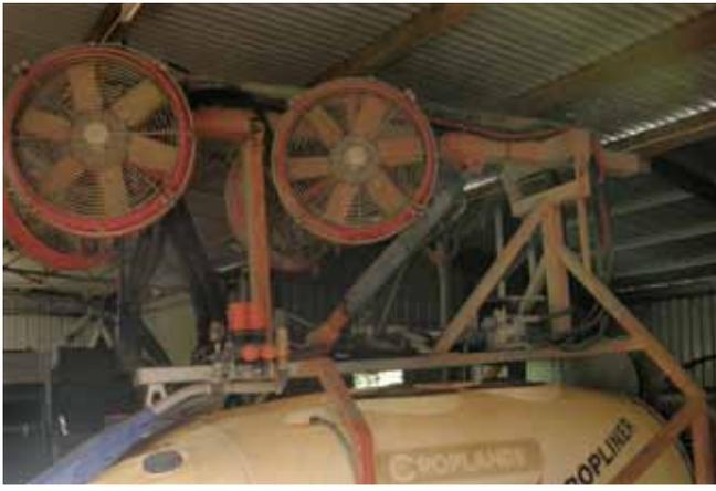
i) *Folded tower fans on top of the air blast sprayer .*
