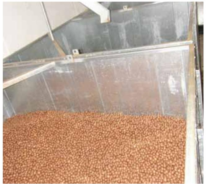
m) *Shallow bed drying/curing system*
