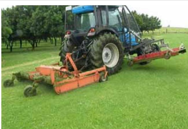
***The under tree mower can be raised for turning and transporting***
